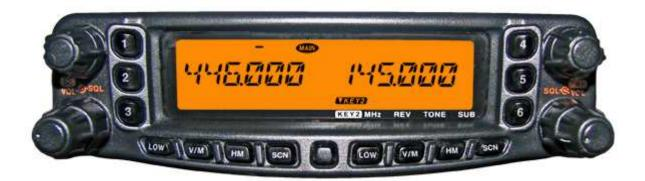
The **FT–8900R** is a ruggedly-built, high quality Quad Band FM transceiver providing 50 Watts of power output on the 29/50/144 MHz Amateur band and 35 Watts on the 430 MHz band.
