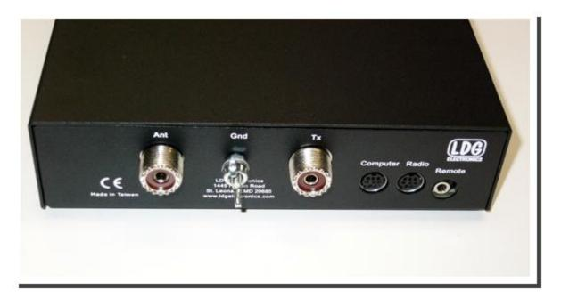
ANT connector: Connect the 50-ohm coax antenna feedline to this standard SO-239 connector.
