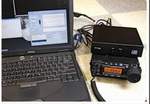
The YT-100 monitors the **Computer** port for activity before beginning any tuning cycle. Only when the CAT line is idle for a period of time will the YT-100 take over control of the CAT line in order to
