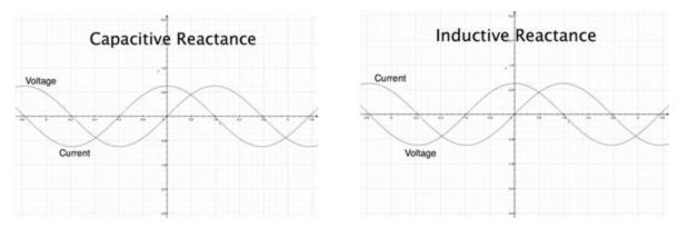
The output circuit of a transmitter consists of inductors and capacitors, usually in a series/parallel configuration called a "pi network". The transmission line can be thought of as a long string of capacitors and inductors in series/parallel, and the antenna is a kind of resonant circuit. At any given RF frequency, each of these can exhibit resistance, and impedance in the form of capacitive or inductive "reactance".
